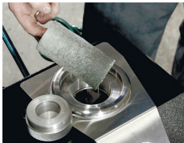
Fig. 6. Filter element after the first flushing cycle.
