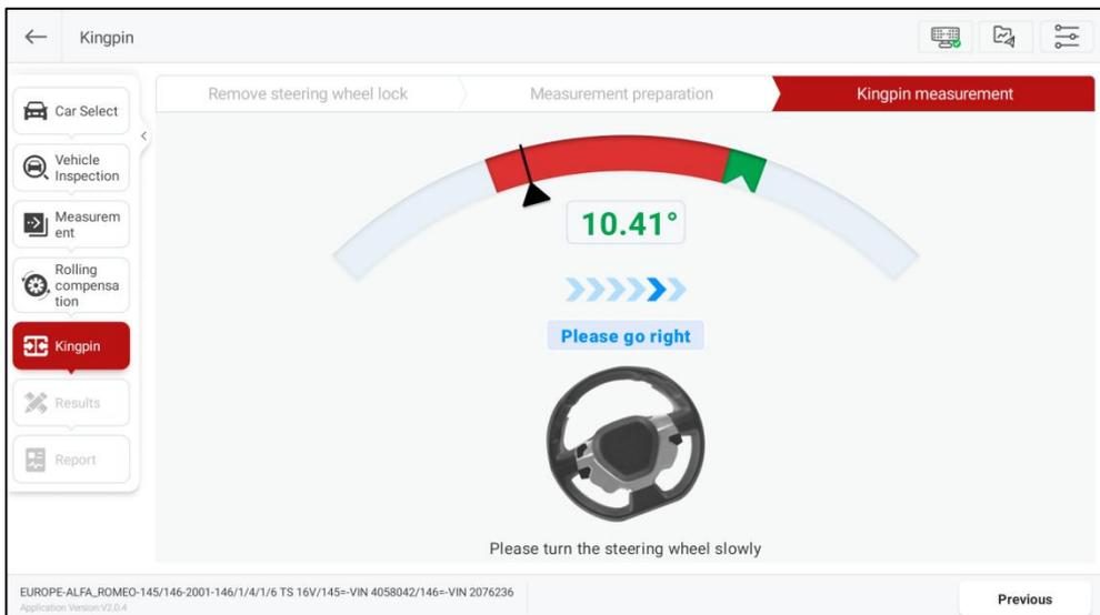
4) According to the system prompt, return the steering wheel to its initial position.
