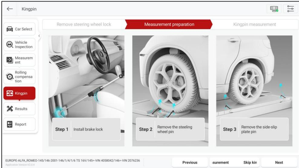
After the preparation is completed, click [Next] to enter the “Kingpin Measurement” interface.
