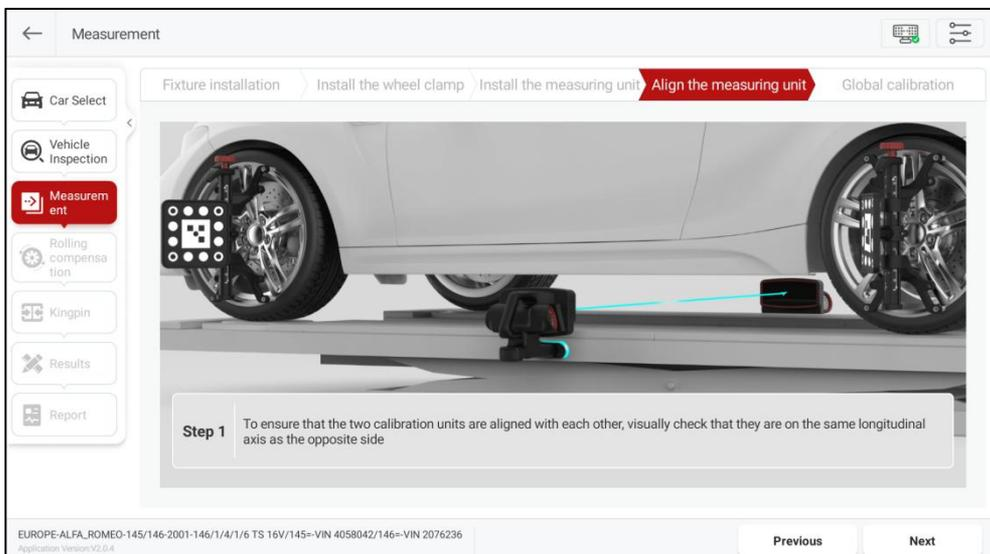
After the clamps and measurement units are all installed, the indicator lights on the measurement units flash blue quickly, indicating that the measurement units are searching for the ST13 intelligent link terminal. The indicator lights then flash blue slowly, which indicates the device is networking internally. When both measurement
