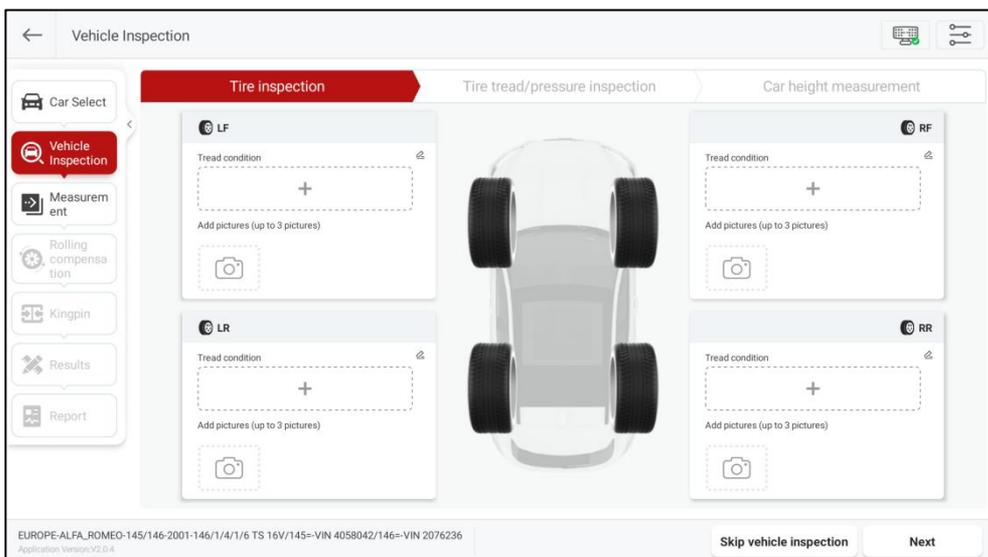
Complete relevant vehicle inspections such as the vehicle tire inspection, tread and tire pressure inspection, and car height measurement, then click [Next] to enter the
