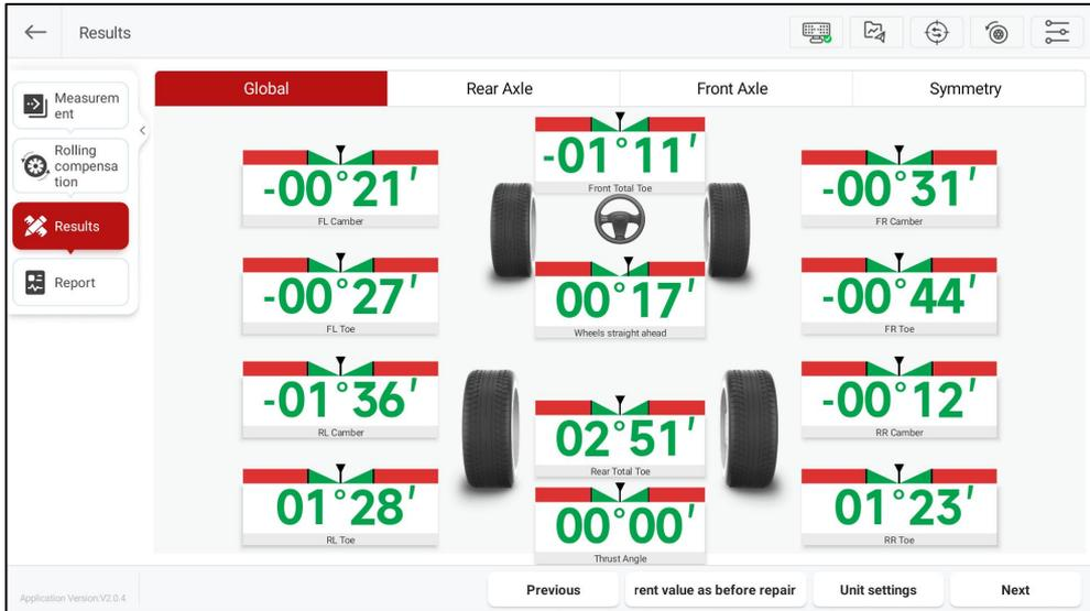
Save the measurement results before maintenance. The measurement results will be updated in real time after the maintenance is completed. Click [Next] to save the current measurement results and enter the “Inspection Report” interface.
