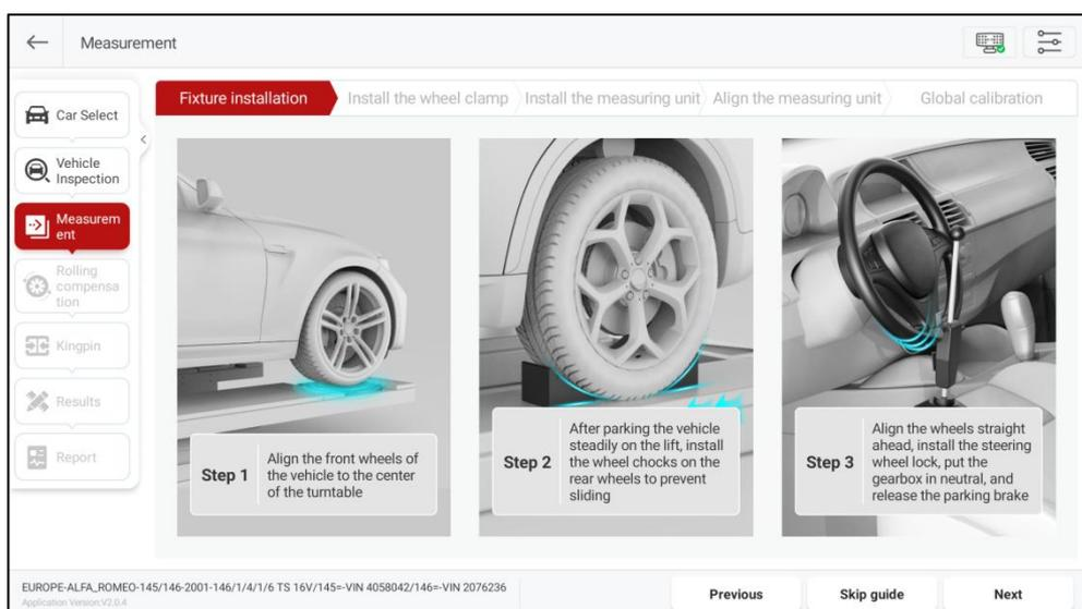
Click [Fixture Installation] and install the relevant fixtures according to the on-screen
