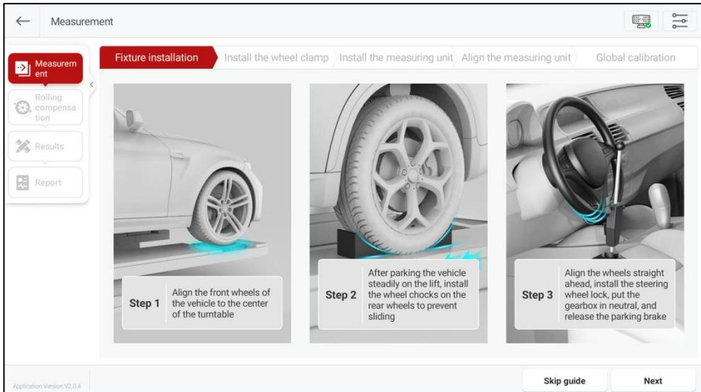
Follow the on-screen instructions to complete the steps such as fixture installation, clamp installation, measurement unit installation, measurement unit alignment, and global calibration. After completing the measurement preparation, click [Next] to enter the "Rolling Compensation" interface.
