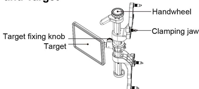
Note: The handwheel is used to adjust the height of the clamping jaw.
