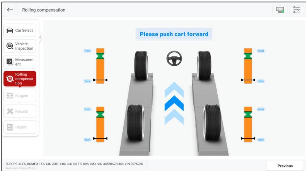
When the interface prompts “Rolling compensation completed”, the rolling compensation is complete and it automatically enters the “Measurement Results” interface.
