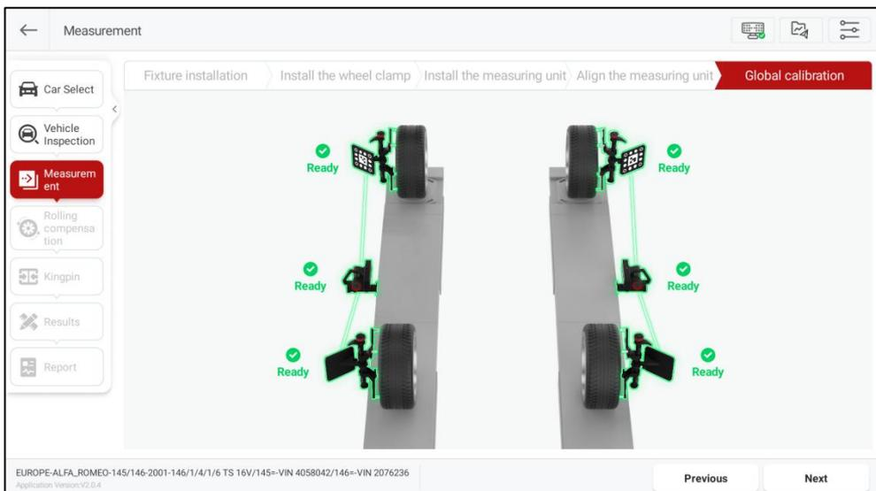
After the device installation is complete, click [Next] to enter the “Rolling Compensation” interface, and push the vehicle according to the prompts on the interface and complete the rolling compensation.
